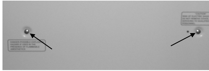
Figure 4 – Middle Rear Panel Screw Locations
